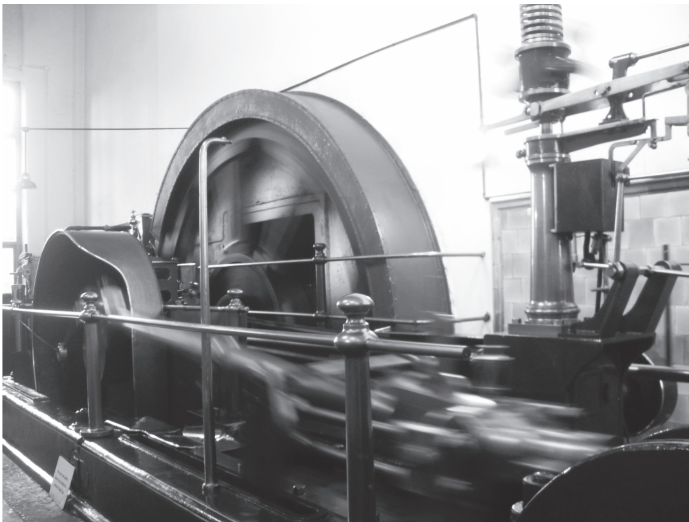
The historic steam engine Peace at Queen Street Mill, built in 1894, running and driving original looms in Autumn 2015.
